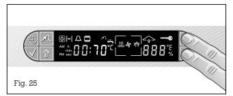
Using the core temperature sensor, during the cooking process you can measure the core temperature of the food you are preparing exactly between 1°C and 99°C. The sensor measures the temperature in the interior of the meat. It indicates when the set core temperature has been reached and the meat has been cooked to satisfaction.
